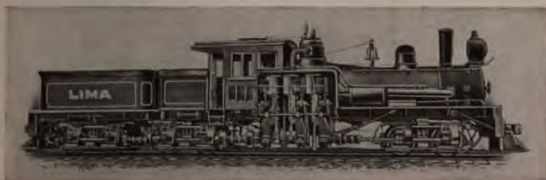
FIG. 88. — A Shay Geared Locomotive.
